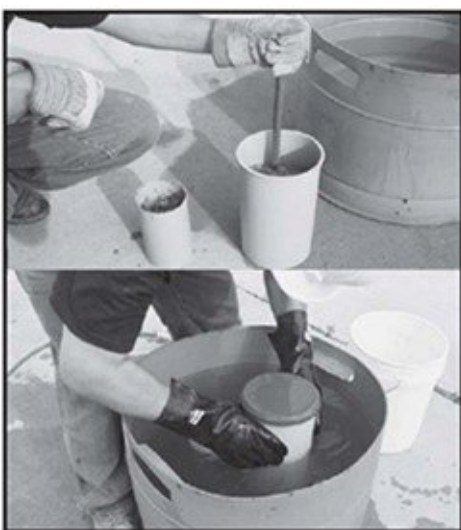
Making Concrete Cylinders 1930s
