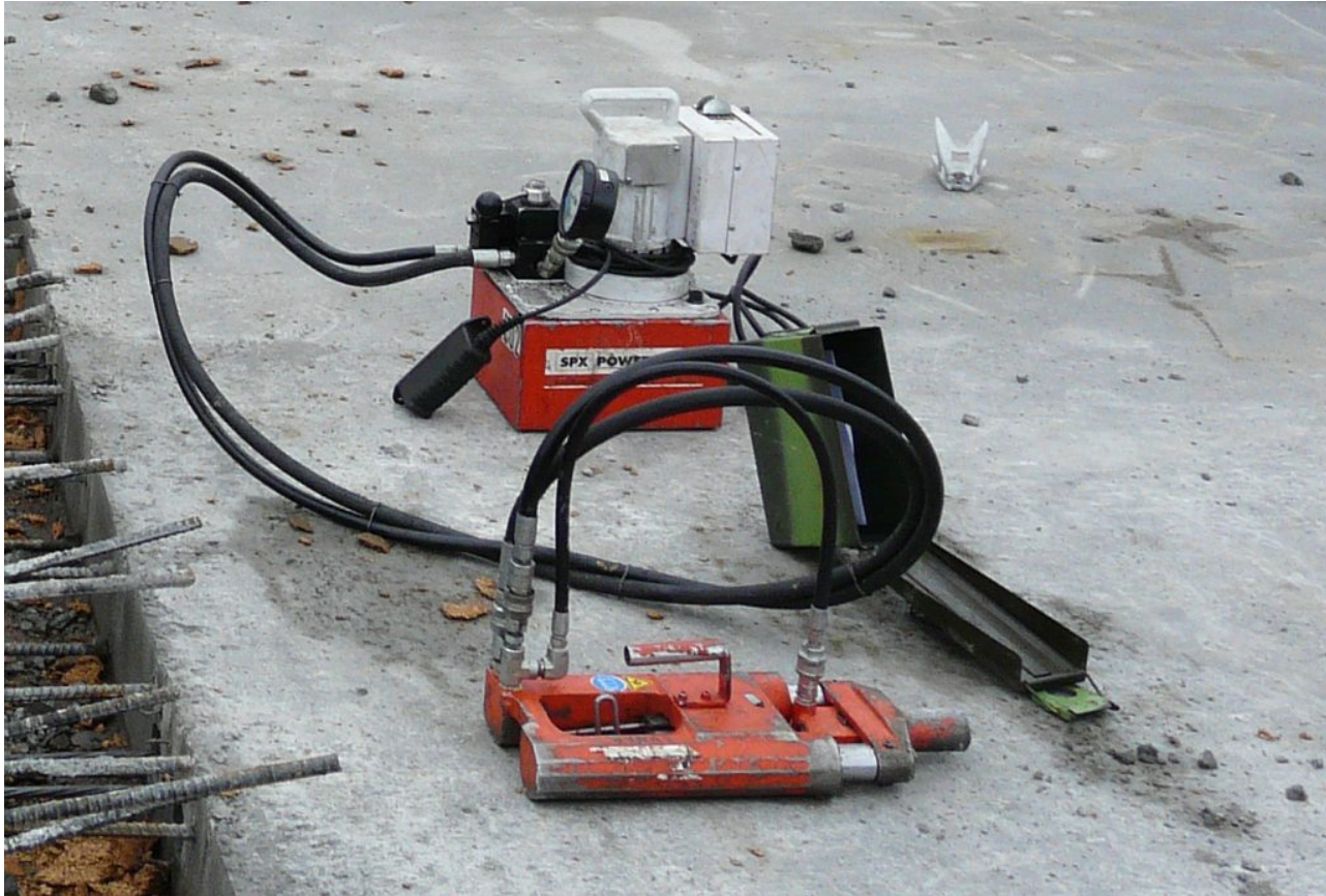
Post-tensioning Hydraulic Jack
