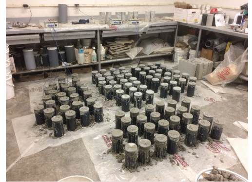
Test cylinders being cured in laboratory
