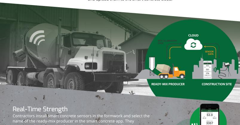
Contractors install smart concrete sensors in the formwork and select the name of the ready-mix producer in the smart concrete app. They can then select the name of the mix from the list of Smart™ mixes to obtain and share real-time concrete temperature and strength data on the job site. This information helps contractors optimize critical operations such as formwork removal, post-tensioning, and opening roads to traffic.
