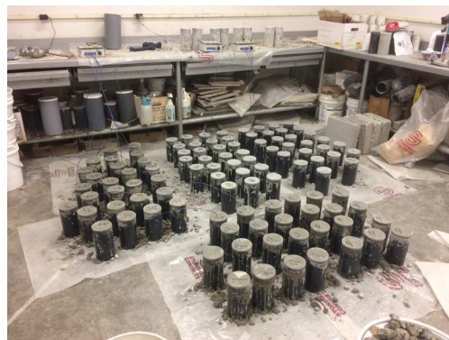
Test cylinders being cured in laboratory
