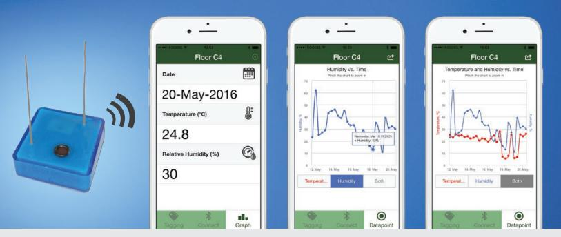
**Giatec BlueRock<sup>TM</sup>** is a rugged waterproof sensor for wireless monitoring the relative humidity and temperature of concrete from fresh stage to hardened stage.
