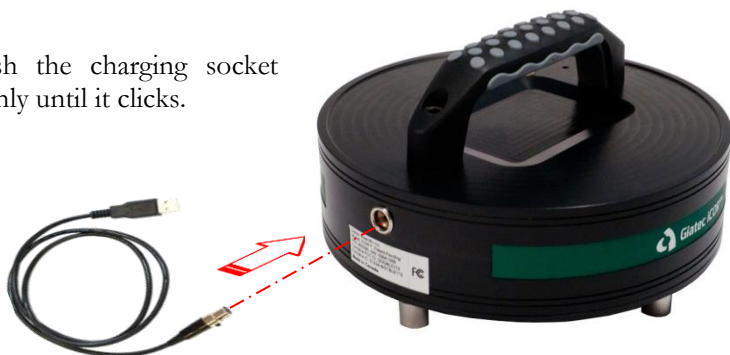
Figure 13. Charging Giatec iCOR™ device.
