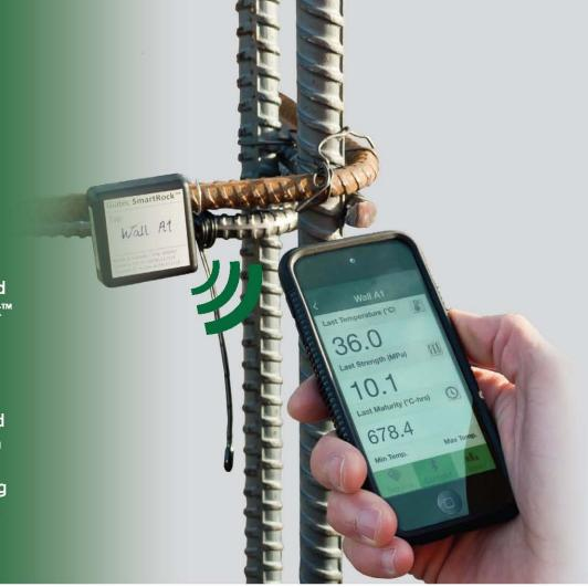
SmartRock™ helps monitor temperature variations in fresh concrete as well as optimize removal time of formwork.
