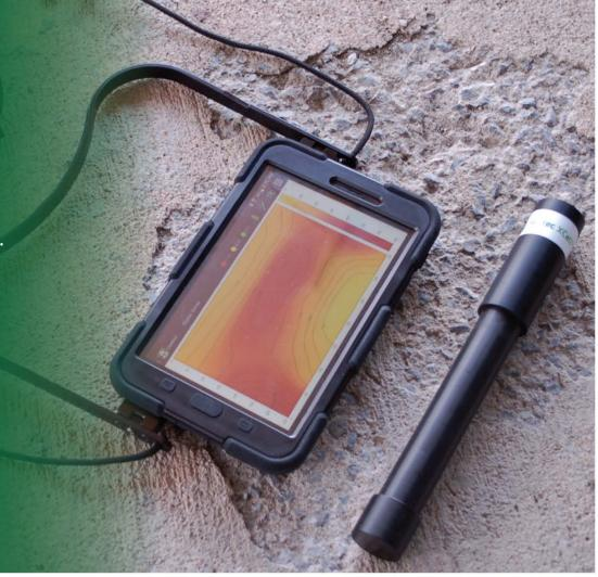
XCell™ makes half-cell potential mapping more efficient and accurate while significantly cutting from the labour and maintenance cost.
