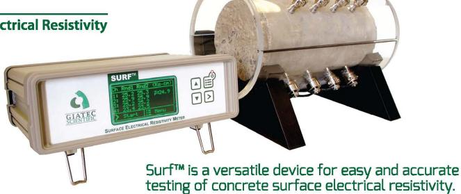
Giatec Surf™ is a laboratory test device for rapid, easy and accurate measurements of the surface electrical resistivity of concrete, based on the four-probe (Wenner-Array) technique. Surf™ utilizes a patented technology to measure resistivity values automatically around the concrete specimen using four channels of a 4-probe array (located at 90° from each other). The data monitor software can be used to perform the test and generate reports.
