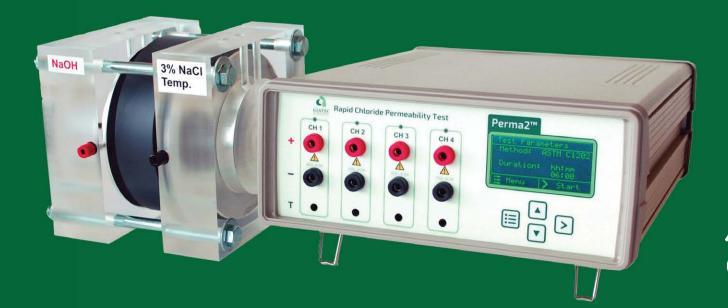
Perma2™ is an accurate device for testing the permeability of concrete based on ASTM and AASHTO standards.
