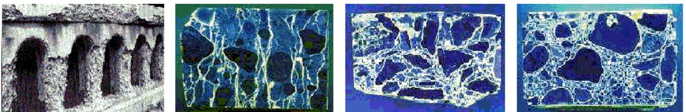
*Typical example of concrete cracked*      *Surface parallel cracks in a Russian concrete*
