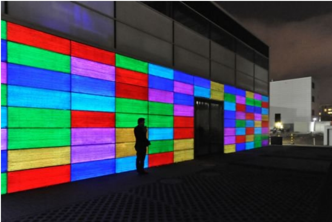
Wall made of LUCEM's transparent concrete
