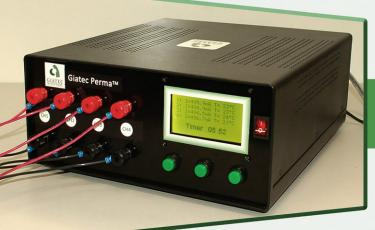
Perma<sup>™</sup> Concrete Permeability Measurement
