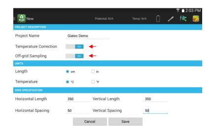
The app automatically corrects potential values for temperature variation. If you do not want the values to be corrected, Turn Off the Temperature Correction feature.
