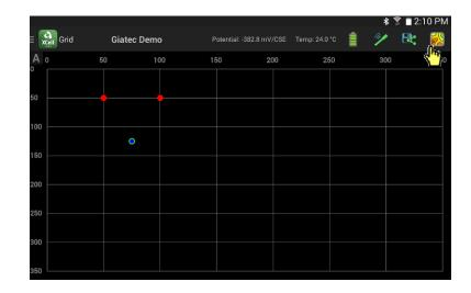
Similar to on-grid data points, the user can re-test any previously tested location. To do so, simply move the probe to the location you want to re-test. Double click on the associated data point. A window will appear where you can select to discard any previously saved value, or replace it with the new value.
