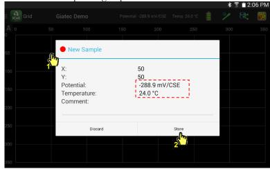
After pressing the store button, the recorded data will be assigned to the grid point. Tested points are indicated with red bullets on the screen. The red bullet with a green margin is the last recorded point.
