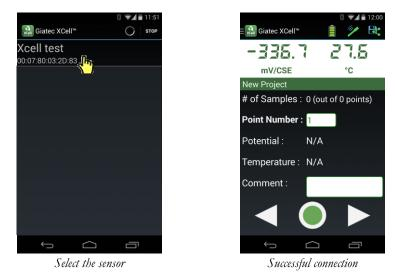
Step 5- Move the probe on the pre-defined grid over the surface of concrete. Wait for the potential value to become stable. As soon as the potential value is stable, press the Green Circle to save its value.
